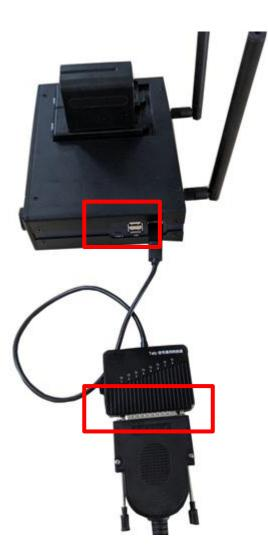
TALLY Signal Universal Converter can be connected to any Type-A port on side of the main station by converter.
