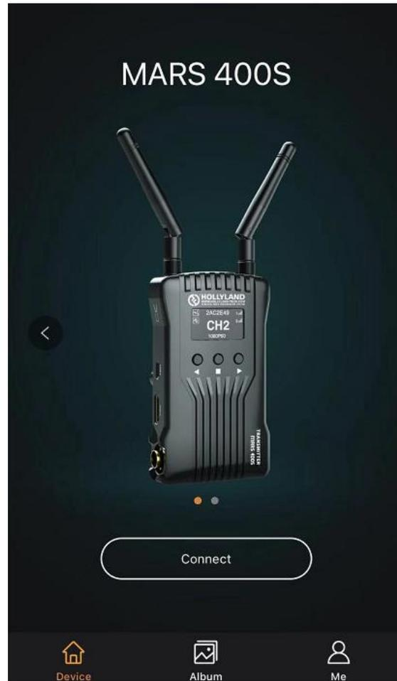
1. Click Connect button to connect device in Device
