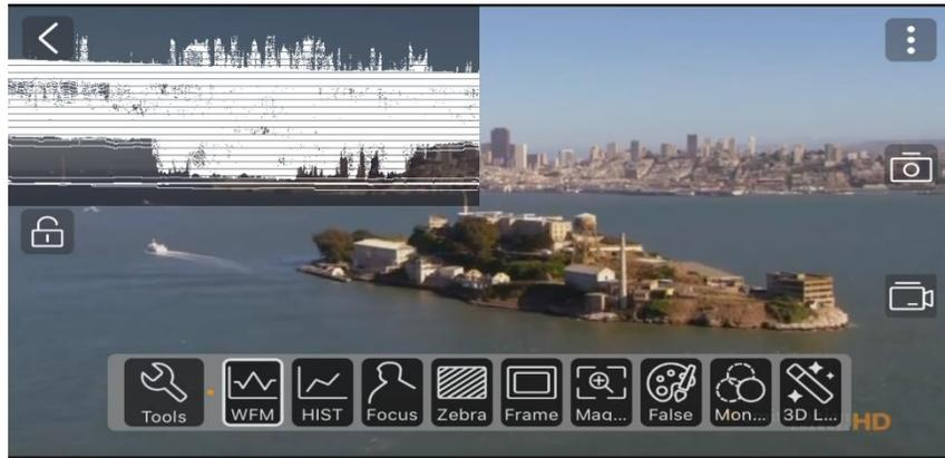
Long press the button to adjust WFM
