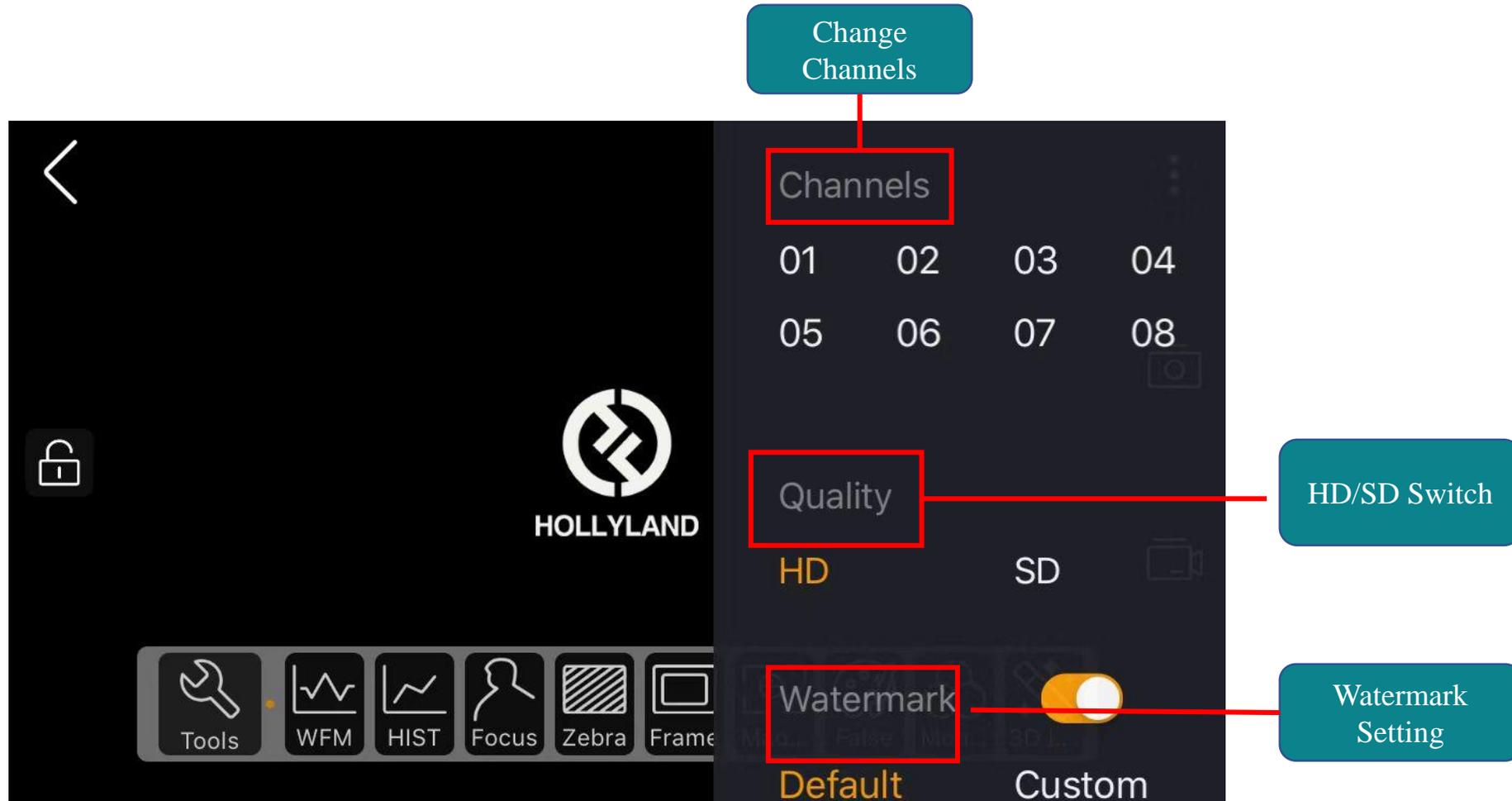
The image shows a screenshot of the HOLLYLAND app's control interface. A dark overlay menu is open, displaying various settings. Three callout boxes with red lines point to specific features:
